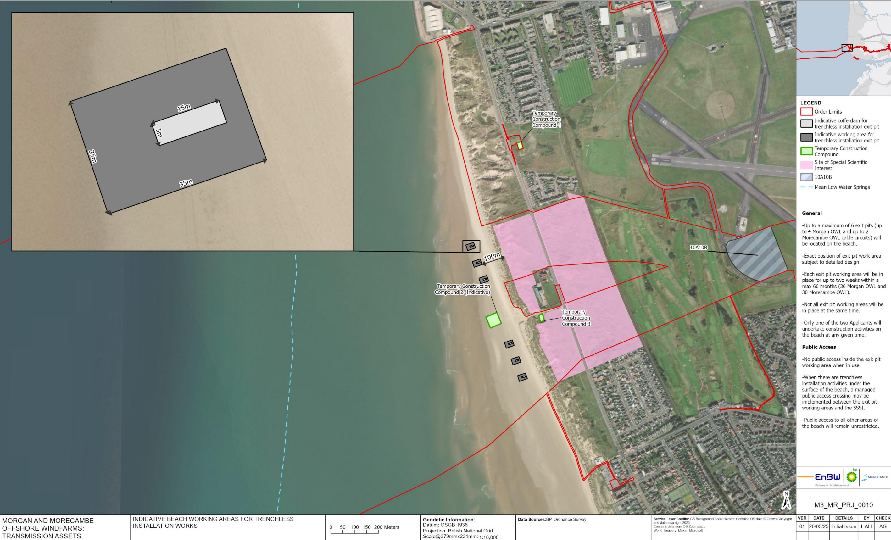
Figure 3: Indicative Beach Working Areas for Trenchless Installation Works
